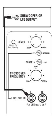
If your receiver/processor does not contain a Dolby Digital or DTS processor but has subwoofer outputs:
